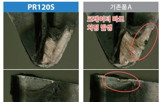
절삭조건 : Vc = 150 m/min, ap = 1.0 mm, f = 0.08 mm/rev, Wet SUS316L DCGT11T304 타입
